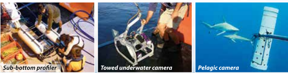
The expedition used a multi-beam sonar, sub-bottom profiler, pelagic cameras, baited video stations, sediment grabs, box cores, benthic sleds, and conductivity, temperature and depth instruments (CTD). The baited mid-water stereo video rigs identified 38 species of sharks and fishes, establishing a baseline for the mid-water assemblage that can be used in the future.
